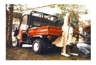
five-gallon buckets for decontamination. Each rig is also fitted with vacuum/volume system to extract soil-gas and groundwater samples from the subsurface. Furthermore, each probing unit carries a complete set of tooling with multiple back-ups to enable our field crews to immediately respond to any changes to the anticipated scope of services. All of HLI's trucks contain firstaid kits, fire extinguishers, and cellular phones to augment site-specific Health
